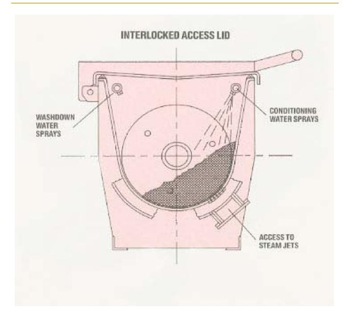
The SCS achieves excellent moisture penetration due to the intimate contact between the product and the process steam / fluid and the elimination of air pockets which act as an insulator.
